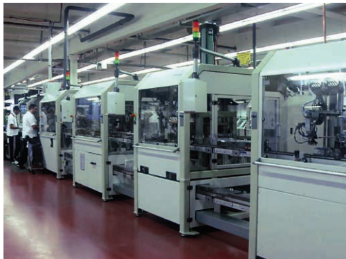
Highly automated production line for PV module junction boxes
